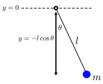
The kinetic energy of an oscillating pendulum is  $K(t) = \frac{1}{2}m\dot{s}^2 = \frac{1}{2}ml^2\dot{\theta}^2$ , and the potential energy is U(t) = mgy, where  $y = -l\cos\theta$  is the height of the particle (where I've called the height of the pivot y = 0). Show that the total energy E = K(t) + U(t) is a constant, independent of time.
